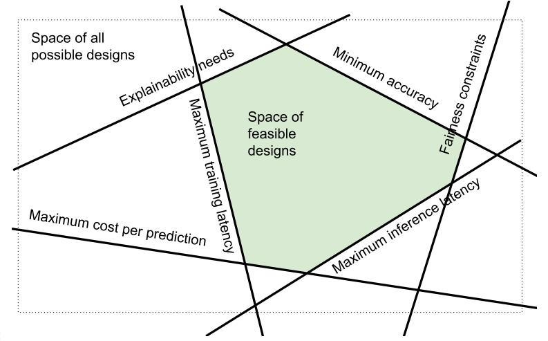
Design space exploration: The space of all possible designs (dotted rectangle) is reduced by several constraints on qualities of the system, leaving only a subset of designs for further consideration (highlighted center area).
